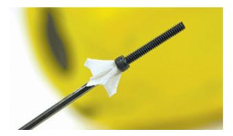
Always have a problem with getting the socket-head bolts into those hard-to-reach spaces? Even though the socket-head bolts do hold on better than a Philips or screwdriver head, they tend to let the bolt fall off just before you can get it started. That's where this trick is really going to save your day! Add a little piece of paper towel to the end of the ball driver and press it into the socket head of the bolt. You will find that this holds better than a magnetic head driver.
